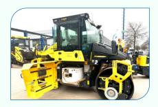
03 Z240 Electric single drum roller BOMAG BW 211/213-e
