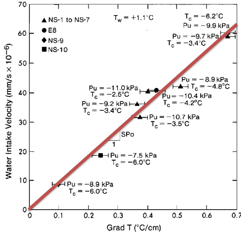
FIG. 1. Relation between water intake velocity and temperature gradient across the active system at the formation of the final ice lens.
