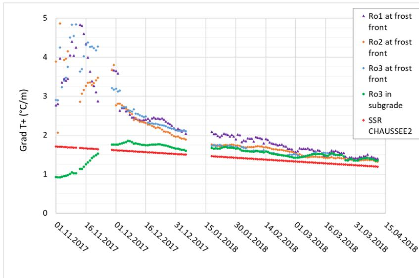
Figure 25: Thermal gradient according to time at Røros test site for winter 2017-18
